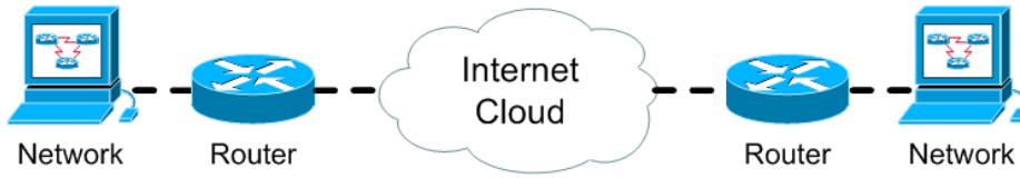
Figure 12.5. Router connections to the Internet cloud
